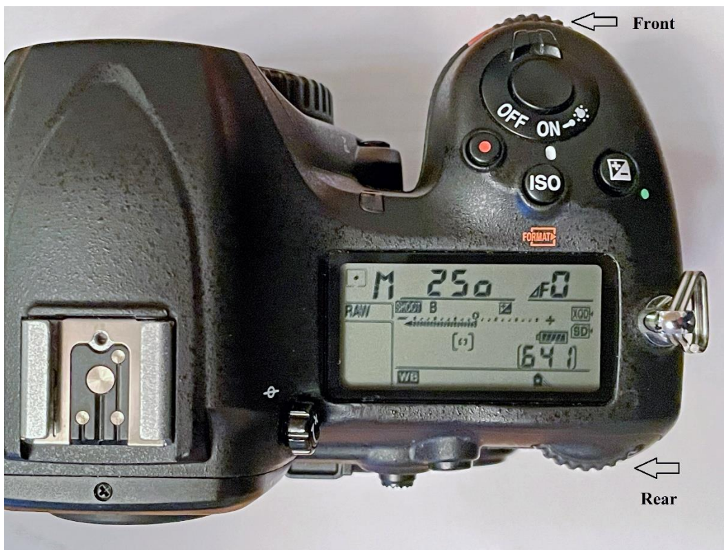
Fig. 1. The rear and front spin selectors as well as the small monitor (referred to as the control panel in the Nikon manuals). The left spin selector is to the left of the flash shoe (not shown here).
