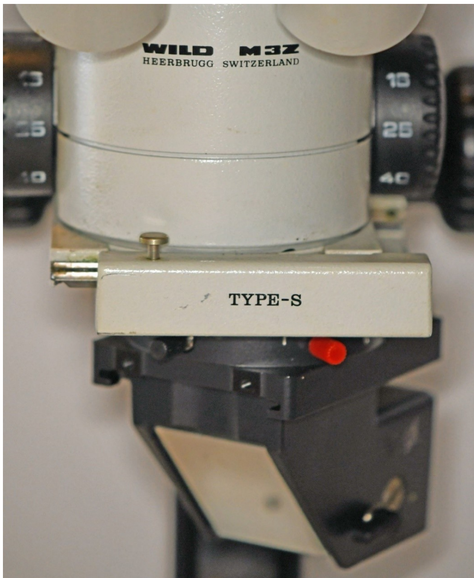
Fig. 6. An oblique viewer (type 404233) by Wild Heerbrugg. Our Wild M3Z is equipped with a Type S holder which is capable of providing a single light beam (see below, Microscope photography ).
