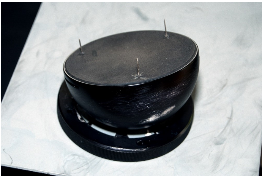
Fig. 4. A turntable designed for small specimens often used with stereomicroscopes. Note that one can drill holes and attach needles for keeping a petri glass or a specimen in place during rotations (and at the same time place a black background photo).
