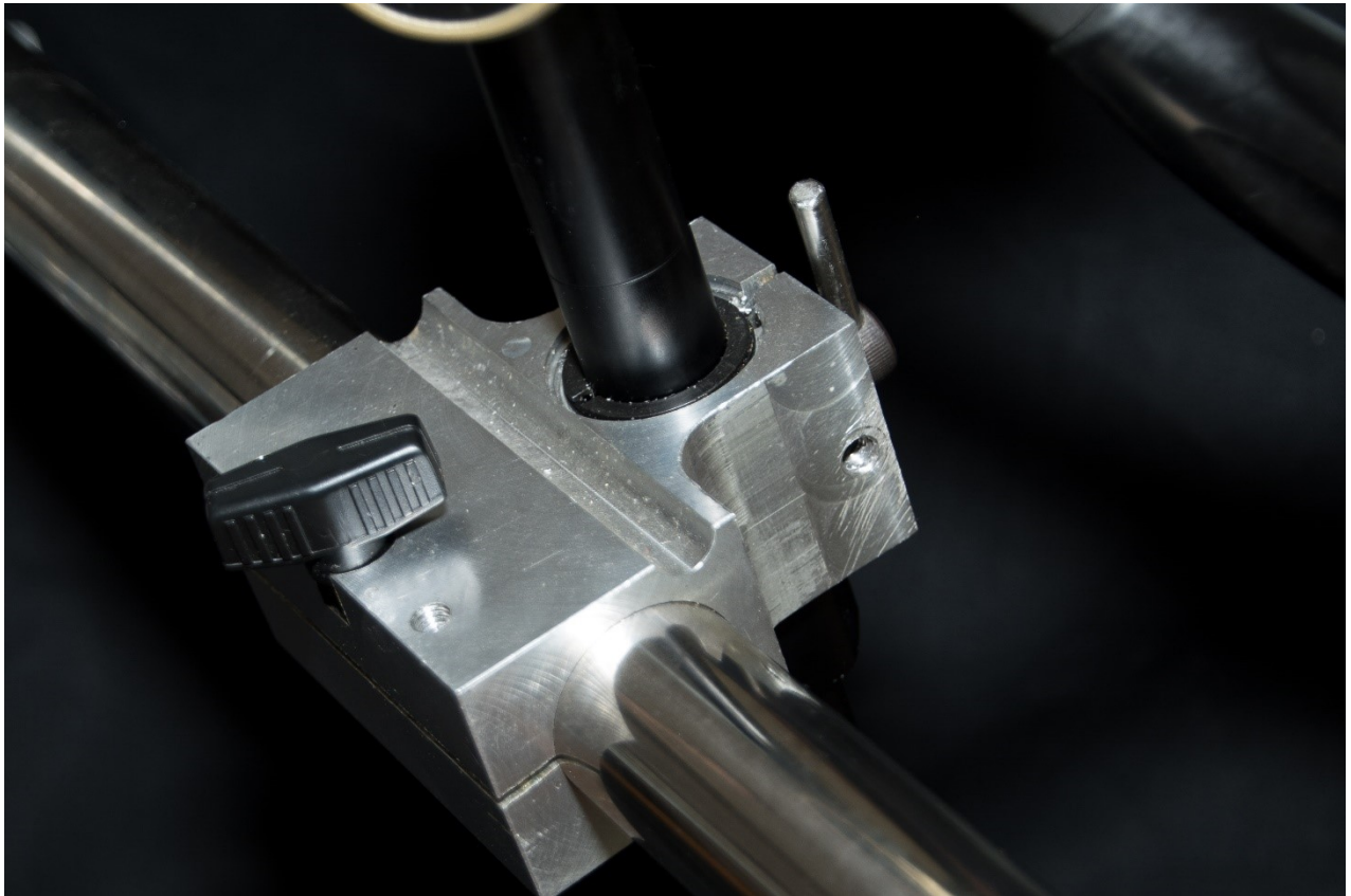
Fig. 3. This aluminium block can (after the release of its two locking mechanisms) be moved horizontally and rotated around the horizontal pipe (which in turn can be moved up and down and around the vertical scaffolding pipe).
