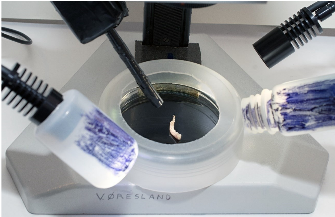
Fig. 106. Plastic beakers and bottles can be cut to fit the light source or surround the object. A Pasteur pipette and black electrical tape can be used to make different-sized spotlight which is useful to light up hollows.
