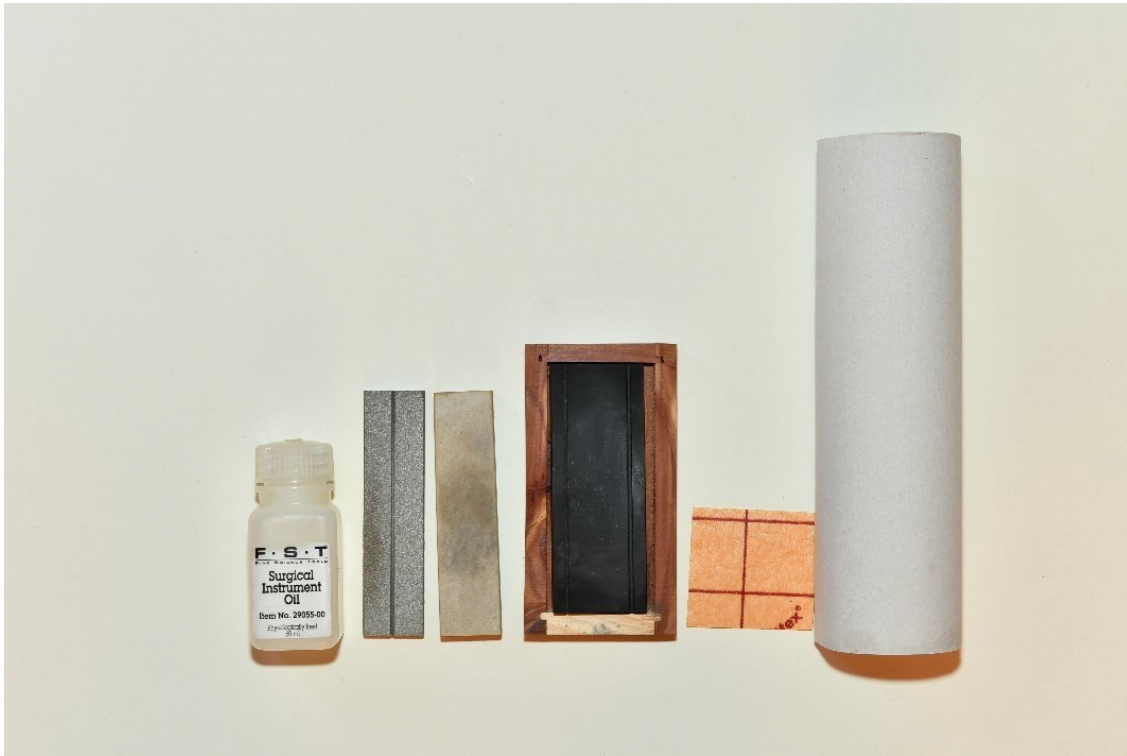
Fig. 101. Oil and sharpening tools. Note that the final sharpening is made on paper.
