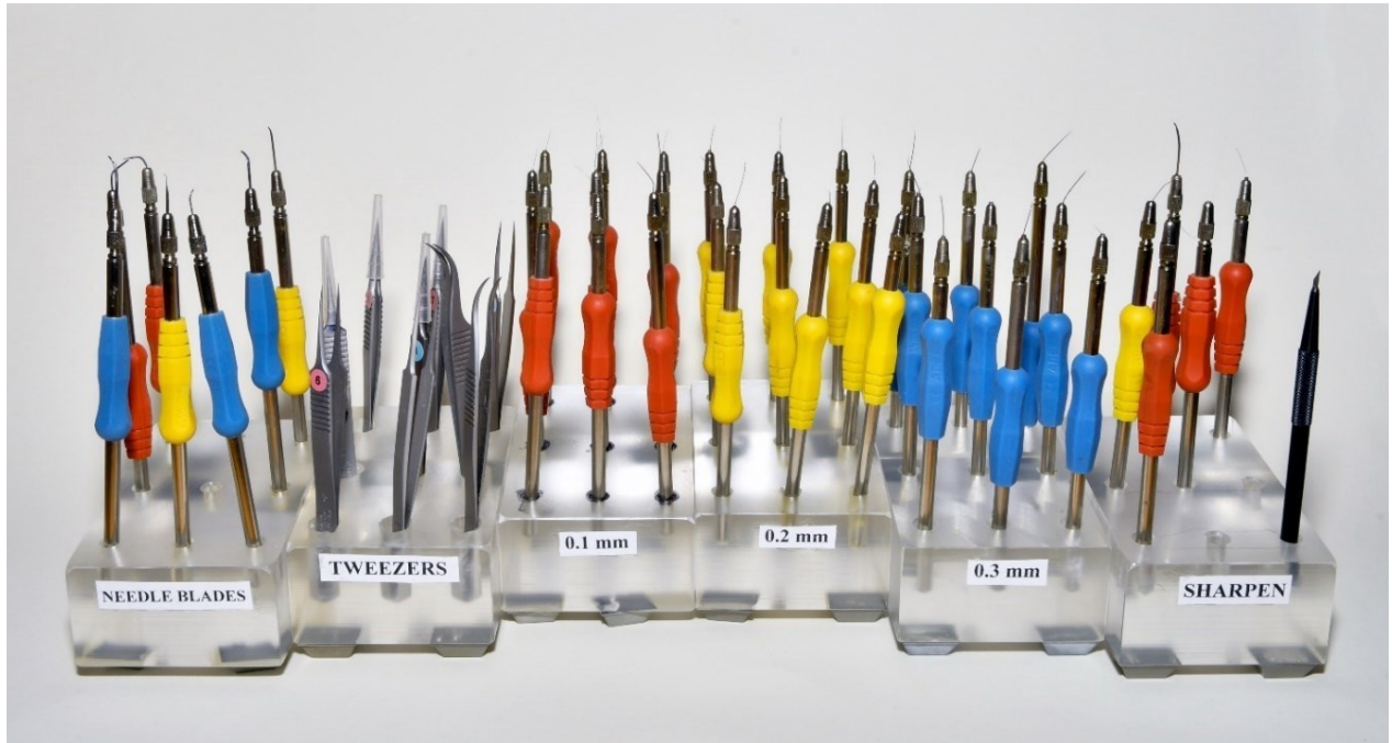
Fig. 104. Keep all dissection tools in separate Plexiglas® holders (or original boxes) that can be placed close to the microscope. Reserve one or two holders for tools that need to be sharpened.
