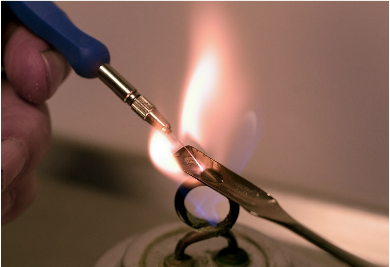
Fig. 103. Sharpening of a tungsten wire in melted \text{NaNO}_2 .
